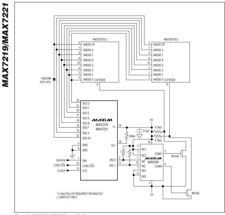
Figure 2. MAX7219/MAX7221 Driving 2.3in Displays
