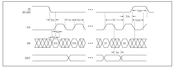
Figure 1. Timing Diagram
