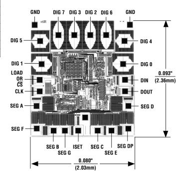
TRANSISTOR COUNT: 5267 SUBSTRATE CONNECTED TO GND
